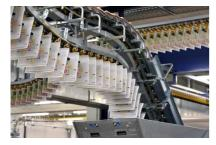
In terms of hardware, the mailroom at a Swiss printing plant has been completely equipped with "reference clamp technology" for the first time, which can be used to address and track each individual newspaper copy with its insert collection.
